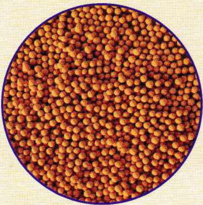
▲ MOL-SIEVE 4A in Spheres form
