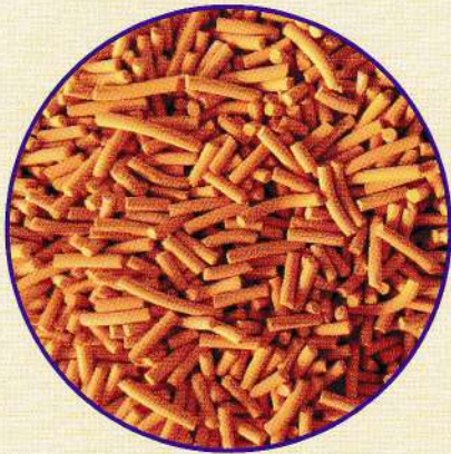
▲ MOL-SIEVE 4A in pellets form
